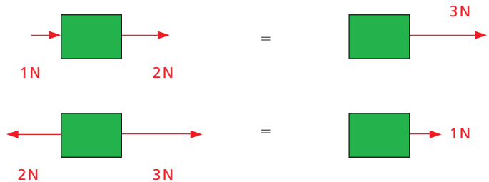
Figure 7.3 The resultant of forces acting in the same straight line is found by addition or subtraction.
