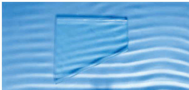
Figure 25.7a Waves are refracted at the boundary between deep and shallow regions.
