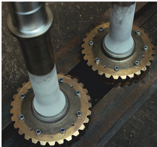
Figure 19.1 'Shrink-fitting' of axles into gear wheels
