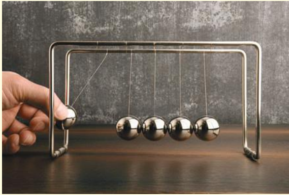
Figure 14.5 Newton's cradle is an instructive toy for studying collisions and conservation of energy.
