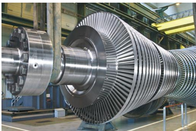
Figure 15.6 The rotor of a steam turbine
